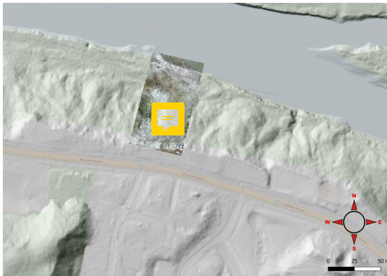
Figure 7: Drone imaging of the 2019 landslide layered on LiDAR digital elevation model of Riverside Avenue
