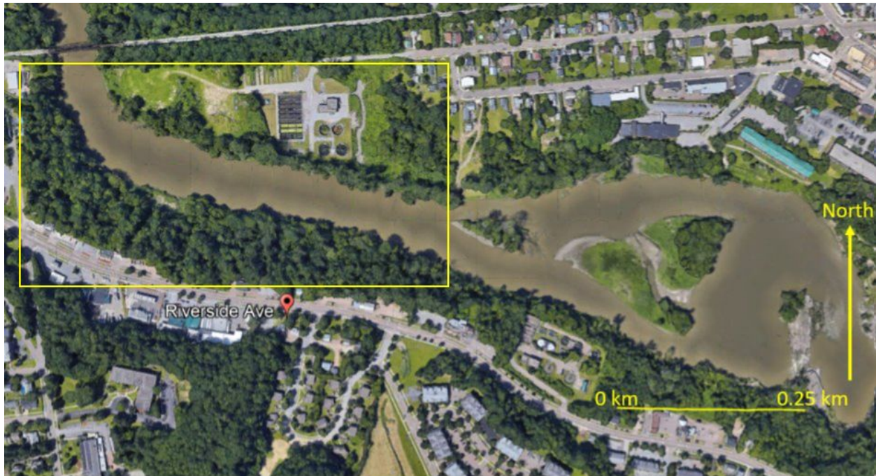
Figure 4: This image of Riverside Ave shows the extensive development and impervious surfaces built on the edge of a 76m high slope leading to the river. The yellow rectangle represents our study area. Photo sourced from Google Maps, 2020.
