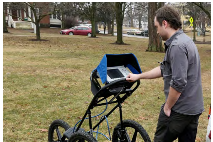
Brennan Gauthier , a 2010 graduate of the UVM Historic Preservation Program who now serves as a Senior Archaeologist in the Environmental Section of Vermont Agency of Transportation demonstrated how portable ground penetrating radar units may assist with archaeological site surveys as a guest speaker in UVM's HP 304 Contemporary Preservation Planning and Policy seminar.
