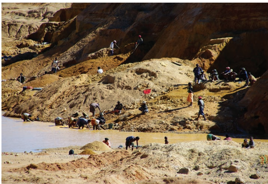
Image 2. Secondary deposit alluvial mining activity near Ilakaka, Madagascar. Diversion of watercourses, slope instabilities, and scarring of landscapes are the main environmental impacts.
