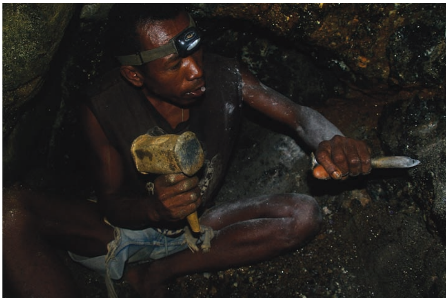
Image 3. Underground mining in a primary corundum deposit. Chiseling in such mica-rich layers presents an important environmental health risk for workers due to resulting dust that contains fine silicate particles.
